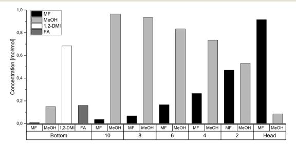
Molar ratios of MF, MeOH, 1,2-DMI and FA in the reboiler, at the trays and in the column head of the reactive distillation column after 740 min.
