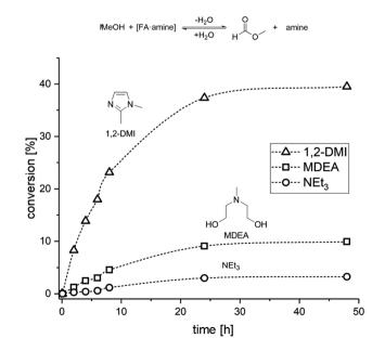
Fig. 3 Time/conversion profiles for the esterification of FA to MF with selected amines in a closed vessel at 60 °C ( $V_{MeOH}$  = 2 mL;  $n_{FA}$  = 6.5 mmol;  $n_{\text{amine}} = 6.5 \text{ mmol}$ ).
