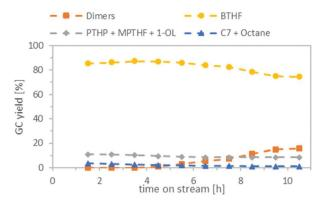
Fig. 8 Continuous flow hydrogenation and deoxygenation of a FFA solution (0.25 mol L<sup>-1</sup>) in cyclohexane. Conditions: Catalyst bed 1<sup>st</sup> reactor: 1 g Ru/C, 50 °C, WHSV = 2  $h^{-1}$ , catalyst bed  $2^{nd}$  reactor: 1 g Ru/ C + 6 g Amberlyst 36, 150 °C, WHSV =  $0.29 h^{-1}$ , substrate flowrate: 1 mL  $min^{-1}$ , hydrogen flowrate: 50 mL<sub>N</sub> min<sup>-1</sup>, pressure: 80 bar. C7 = n-heptane and 2-methyl-5-ethyltetrahydrofuran.
