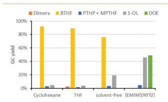
Fig. 5 Influence of the solvent on the deoxygenation of THFA. Conditions: THFA (0.75 mmol), Ru/C (3.75  $\mu$ mol Ru), Amberlyst-36 (9.3 mg, 0.05 mmol H $^+$ ), H $_2$  (80 bar), 150 °C, 6 h, solvent (1.5 mL). [Emim][NTf2] = 1-ethyl-3-methylimidazolium bis(trifluoromethyl-sulfonyl)imide.
