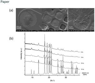
Fig. 3 (a) SEM images of crystals formed in printed droplets on an XRD mesh (10 nL) and (b) XRD patterns for crystals formed in printed 5 and 10 nL droplets showing characteristic peaks for the  $\alpha$  polymorph (calculated reference PXRD patterns for mannitol polymorphs are given in Fig. S2 $\dagger$ ).
