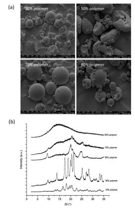
Fig. 6 a) SEM images and b) PXRD patterns of spray dried mannitol with Eudragit polymer (10 to 90% w/w).
