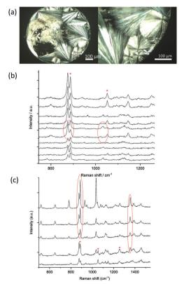
Fig. 1 (a) PLM images of mannitol crystals in a 100 nL droplet printed on a glass slide, (b) and (c) Raman spectra from crystals formed in 100 and 200 nL droplets (the star indicates the band characteristic of the  $\delta$  form and the circle indicates the band characteristic of the  $\alpha$  form).
