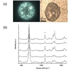
Fig. 2 (a) Images of single droplets on glass (left) and aluminium (right) and (b) Raman mapping results for one single 100 pL droplet on aluminium (stars indicate characteristic bands for the  $\beta$  polymorph).
