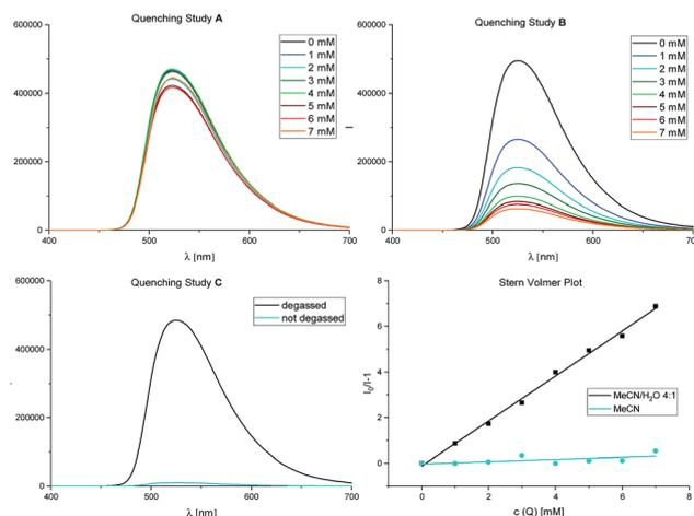
Fig. 2 Stern–Volmer quenching studies. Fluorescence spectra for *fac*-Ir(ppy)<sub>3</sub> (50  $\mu$ M) with increasing amounts of  $\alpha$ -acetoxy acetophenone **1** (0–7 mM) as quencher. Quenching study A: in MeCN; quenching study B: in MeCN/H<sub>2</sub>O 4 : 1; quenching study C: presence of oxygen. For further details, see ESI.†
