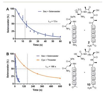
Fig. 1 Rate of model PNA-templated ligation reactions. (A) Ligation of diselenide dimer 2 and selenoester 8. (B) Rate comparison of selenocystine—selenoester ligation and NCL (Cys 10 + thioester 9).
