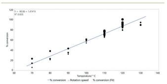
Fig. 9 The linear relationship between temperature and % conversion estimated by <sup>1</sup>H NMR spectroscopy. Line of best fit: y = -90.1 + 1.47xand  $R^2 = 0.935$ .
