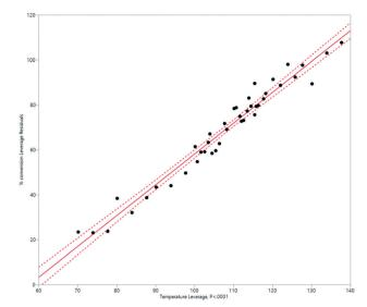
Fig. 10 Modelling the HeRo process, plotting temperature against % conversion estimated by <sup>1</sup>H NMR spectroscopy.
