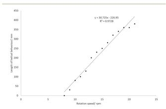
Fig. 7 The effect of rotation speed on the length of the helix at 110
