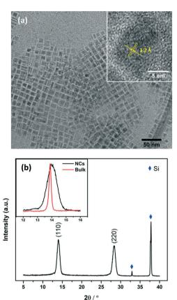
Fig. 2 (a) TEM images of MAPbl<sub>3</sub> NCs stored for over 8 months. The inset is the high resolution TEM of a typical NC. The interplanar spacing was measured to be 3.2 Å, which is consistent with the (220) plane of tetragonal phase MAPbI<sub>3</sub> perovskite.<sup>26</sup> (b) XRD patterns of MAPbl<sub>3</sub> NCs coated on silicon wafer. The inset is the comparison of the (110) peak of MAPbl<sub>3</sub> NCs with that of the bulk film.
