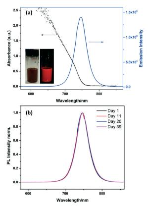
Fig. 3 (a) Absorption and photoluminescence of MAPbI<sub>3</sub> NCs solution in toluene. The insets show the solution under ambient and UV light. (b) PL spectra taken for MAPbl<sub>3</sub> NCs solution over 39 days. The solution was stored in a sealed vial at room temperature in the dark.
