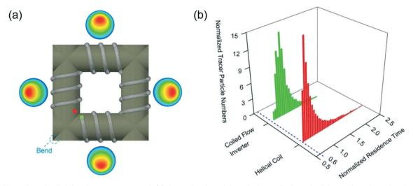
Fig. 4 (a) Illustration of coiled flow inverter reactor with 90 degree bends and the velocity profile in each of the sections. It can be observed that the maximum velocity is shifted towards the direction of the centrifugal force in each of the straight sections. Red and green dots represent the inlet and outlet points, respectively. (b) Comparison of the dimensionless residence time distribution in straight helical reactor and CFIR.
