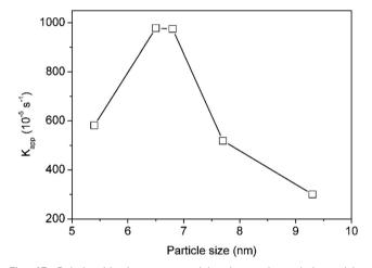
Fig. 13 Relationship between particle size and catalytic activity. Reaction conditions:  $3.3 \times 10^{-5}$  M 4-NP,  $6.6 \times 10^{-2}$  M NaBH<sub>4</sub> and  $2.24 \times 10^{-2}$  $10^{-5}$  g L $^{-1}$  silver nanoparticles at room temperature.
