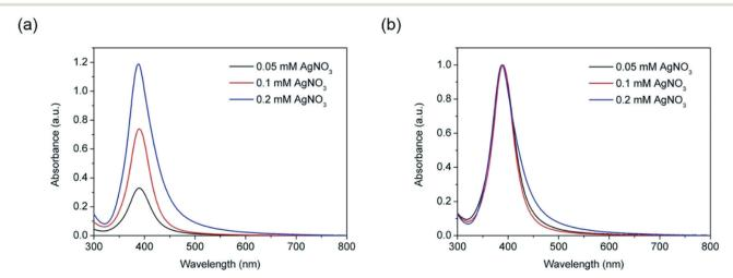
Fig. 3 (a) UV-vis absorbance spectra and (b) normalized absorbance spectra for Ag nanoparticles synthesized with different concentration of AgNO<sub>3</sub> at a constant NaBH<sub>4</sub>: AgNO<sub>3</sub> molar ratio of 11:1. SHR, helix diameter: 10 mm, pitch distance: 1/π cm, length: 1 m, 0.03" ID. The total flowrate is 0.5 mL min<sup>-1</sup>, residence time: 54 s.
