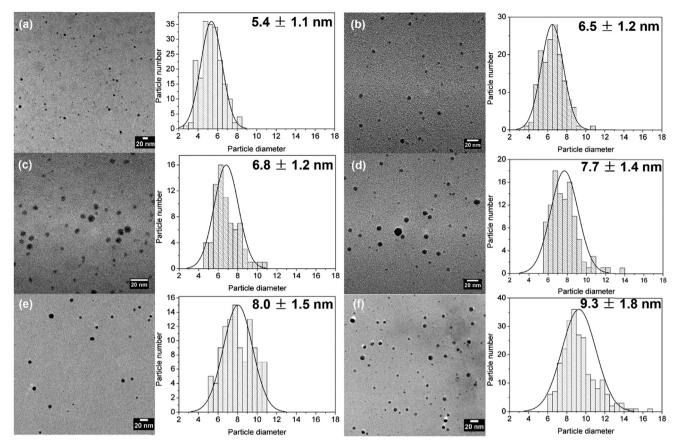
Fig. 10 TEM and particle size distribution of (a) seed particles, (b) AG-0.5 mM particles, (c) AG-1 mM particles, (d) AG-1.5 mM particles, (e) AG-1.75 mM particles and (f) AG-2 mM particles. Reaction conditions as in Fig. 9.
