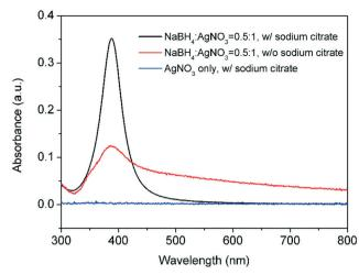
Fig. 7 Effect of the presence of sodium citrate on the silver conversion (proportional to absorption) and size distribution: 0.05 mM AgNO<sub>3</sub>, 0.025 mM NaBH<sub>4</sub>, and 0.35 mM Na<sub>3</sub>CA, 60  $^{\circ}$ C, residence time of 71 s, CFIR.
