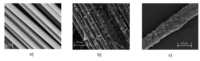
Fig. 4 (a) SEM image of untreated glass fibre roving ( $\times$ 2000); (b) SEM image graphene-based (coated) glass roving ( $\times$ 500); and (c) SEM image graphene-based (coated) glass roving ( $\times$ 1000).
