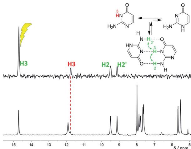
Fig. 3  $^1\text{H}$  NMR spectrum (bottom) and differential  $^1\text{H}$  NOE spectrum (top, irradiation at 14.7 ppm) of isocytosine in DME/DMF- $d_7$  solution at  $-120^\circ\text{C}$  confirming the dimer formation. The signal indicated by a red dashed line is the exchange signal of H3 in the isocytosine monomer.
