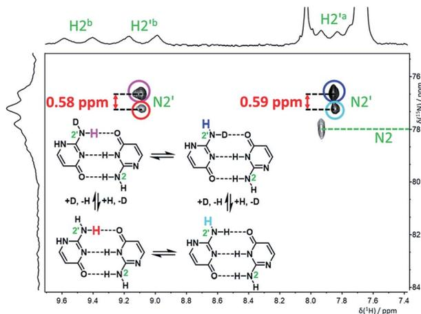
Fig. 4 H,N-HSQC spectrum of  $^{15}\text{N}$ - and partially  $^2\text{H}$ -labelled isocytosine in DME/DMF- $d_7$  at  $-120^\circ\text{C}$ , showing the deuterium-induced isotopic shifts of nitrogen N2' caused by isotope exchange of the hydrogen atoms involved and not involved in intermolecular hydrogen bonding ( $\text{H}2^{\text{b}}$  and  $\text{H}2^{\text{a}}$ , respectively).
