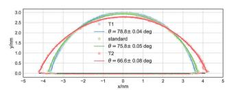
Fig. 2 Points at constant density in the x-z plane for the water droplets simulated using the NH, T1, and T2 thermostats. The solid lines are the best fit to an arc of a circle. The caption reports the values of the corresponding
