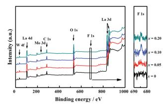
Fig. 2 XPS wide-scan spectra of  ${\rm La_{5.5}W_{0.6}Mo_{0.4}O_{11.25-\delta}F_x}$  ( $x \le 0.2$ ) ceramics.
