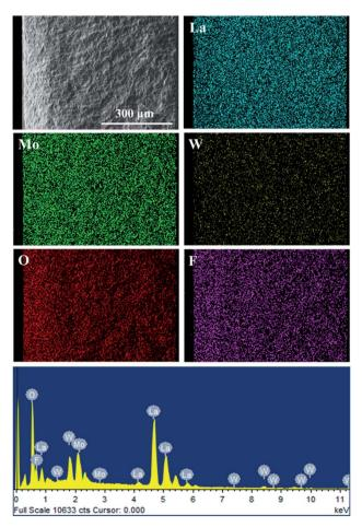
Fig. 3 SEM-EDXS image of the  $La_{5.5}W_{0.6}Mo_{0.4}O_{11.25-\delta}F_{0.05}$  membrane.
