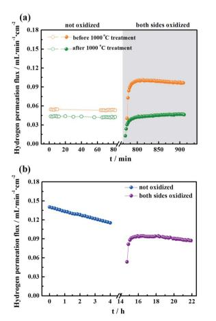
Fig. 10 (a) The regeneration of hydrogen permeation fluxes for the  $La_{5.5}W_{0.6}Mo_{0.4}O_{11.25-\delta}F_{0.05}$  membrane at 950 °C. (b) The oxidization effect on the permeability of the  $La_{5.5}W_{0.6}Mo_{0.4}O_{11.25-\delta}F_{0.05}$ membrane at 1000 °C.
