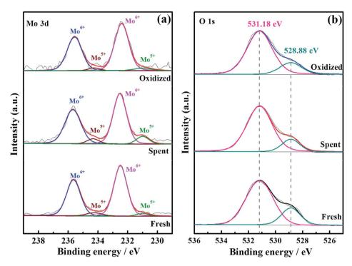
Mo 3d (a) and O 1s (b) XPS spectra of fresh, spent and oxidized  $La_{5.5}W_{0.6}Mo_{0.4}O_{11.25-\delta}F_{0.05}$  membranes
