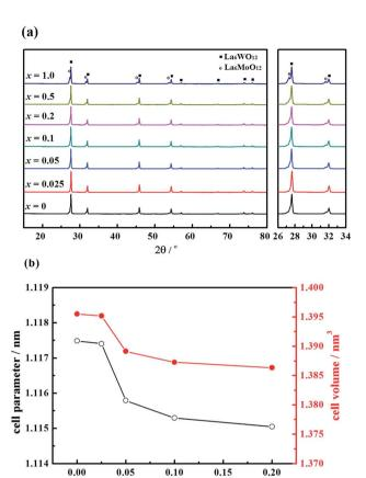
Fig. 1 (a) X-ray diffraction patterns and (b) the cell parameter and the cell volume of the La<sub>5.5</sub>W<sub>0.6</sub>Mo<sub>0.4</sub>O<sub>11.25- $\delta$ </sub>F<sub>x</sub> membranes sintered at 1500 °C.
