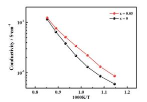
Fig. 6 Conductivity as a function of temperature plotted in the Arrhenius form under a wet (pH<sub>2</sub>O = 0.025 atm) 10% hydrogen in argon atmosphere for LWMF<sub>0</sub> and LWMF<sub>0.05</sub> specimens.
