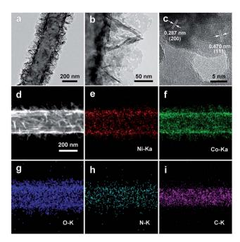
Fig. 3 (a, b) Typical TEM images of NiCo $_2$ O $_4$  nanosheets on carbon nanofiber films at different magnifications; (c) an HRTEM image of NiCo $_2$ O $_4$  nanosheets; (d–i) HAADF-STEM and corresponding EDX elemental mappings (Ni, Co, O, N, C) of NiCo $_2$ O $_4$ @CNFs.
