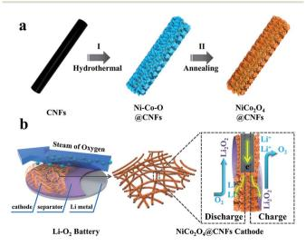
Fig. 1 (a) Schematic illustration of the fabrication of the NiCo<sub>2</sub>O<sub>4</sub>@CNFs cathode; (b) structure of the rechargeable Li-O<sub>2</sub> battery containing this cathode.
