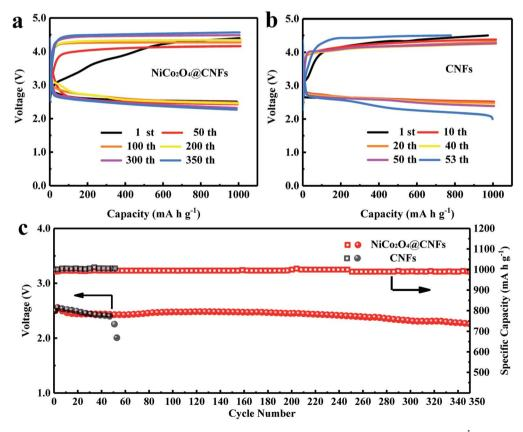
Fig. 5 (a and b) The cycling performance of NiCo $_2$ O $_4$ @CNFs and CNFs cathodes at a current density of 200 mA g $^{-1}$  and a specific capacity limit of 1000 mA h  $g^{-1}$ ; (c) the terminal discharge voltage as a function of cycle number for Li-O<sub>2</sub> batteries with NiCo<sub>2</sub>O<sub>4</sub>@CNFs and CNFs cathodes.
