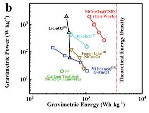
Fig. 6 (a) Initial full discharge capacity and cycle performance limited capacity results of previously reported studies based on oxygen electrodes (blue rhombus: organic binder; black solid circle: binderfree; orange circle: noble metal electrodes); (b) gravimetric energy and power of various oxygen electrodes compared with those of LiCoO<sub>2</sub> (NF: Ni foam; CT: carbon textile).
