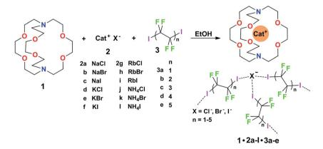
Fig. 2 Starting chemical species 1, 2a-l, and 3a-e and schematic representation of the structural units in corresponding cocrystals  $1\cdot 2a-l\cdot 3a-e$ . A pattern of three XBs around the anion is depicted as it is the by far most common arrangement in the library (it is present in twenty eight of the thirty one X-ray structures).
