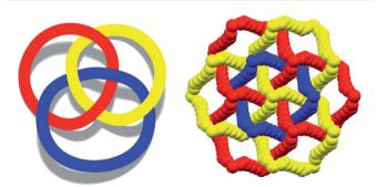
Fig. 1 Left: Schematic view of discrete Borromean ring. Right: Partial view (Mercury 3.8, space-filling) of the three honeycomb nets present in the cocrystal  $1 \cdot 2f \cdot 3d$ . Red, yellow, and blue colours differentiate the three translationally related nets showing Borromean entanglement. Supercations  $K^+ \subset 1$  are omitted for clarity.
