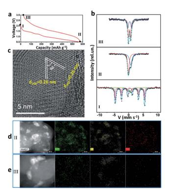
**Fig. 3** (a) Discharge-charge curves of the first cycle at the specific current of 0.2 A g $^{-1}$ ; (b)  $^{57}\text{Fe}$  Mössbauer spectra, (c) TEM image, (d) STEM and (e) EDS mappings of the as-prepared Fe $_3\text{S}_4$  at different states.
