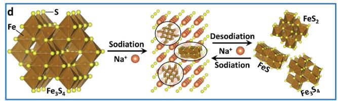
Fig. 4 (a) TEM image, (b) SAED pattern and (c) HRTEM image of the as-prepared  $Fe_3S_4$  at a full charge state after 200 cycles. (d) Schematic illustration of the sodium-storage mechanism in the  $Fe_3S_4$  electrode.
