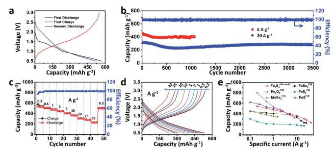
Fig. 2 Electrochemical performance of the as-prepared Fe<sub>3</sub>S<sub>4</sub>. (a) Discharge-charge curves of the first two cycles at a specific current of 0.2 A  $g^{-1}$ ; (b) cycling performances at 5 and 20 A  $g^{-1}$ ; (c) rate capability and (d) discharge-charge curves at various current rates; (e) comparison of the as-prepared Fe<sub>3</sub>S<sub>4</sub> with other conversion anode materials of SIBs.
