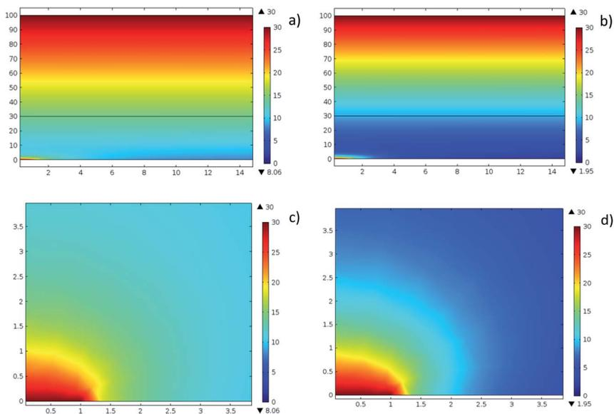
Fig. 5 Salt-concentration distributions in the vertical plane passing through the hole center: hole radius  $1 \mu\text{m}$ , cell half-size  $15 \mu\text{m}$ ; in the upper maps (a, b) the scales along the vertical and horizontal axes are different; the lower maps (c, d) show the magnified vicinity of the hole with the same scaling along both axes. The hole center is in the lower left corner. (a, c)  $\phi_0 = 93$  mV; (b, d)  $\phi_0 = 200$  mV.
