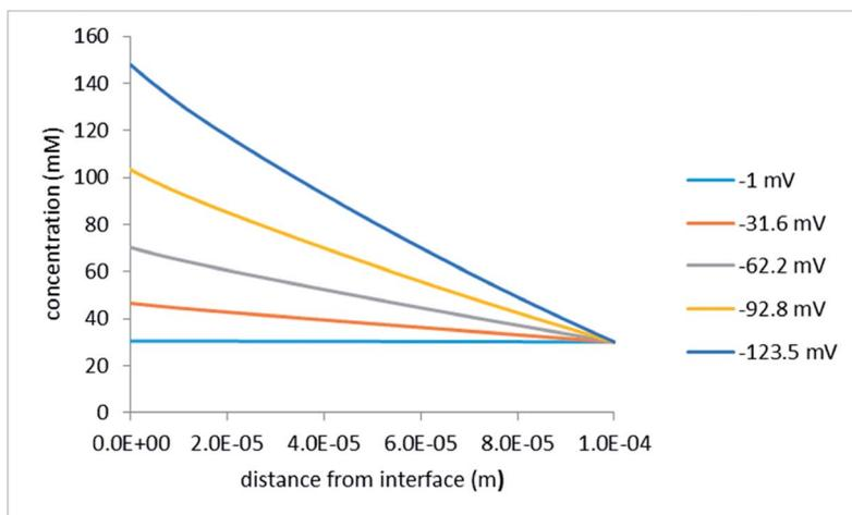
Fig. 9 Concentration distribution along the  $z$ -axis at the upper right cell corner (see Fig. 2); the legend indicates the applied voltages; the half-distance between the hole centers is 15  $\mu\text{m}$ .
