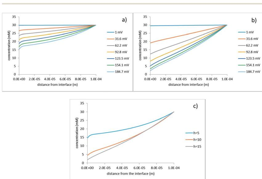
Fig. 7 Concentration profiles along the z-axis at the upper right cell corner (see Fig. 2); (a)  $h = 5 \mu\text{m}$ ; (b)  $h = 15 \mu\text{m}$ ; the legends indicate the applied voltage; (c)  $\varphi_0 = 200 \text{ mV}$ , the legend indicates the half-distance between the hole centers in micrometers.
