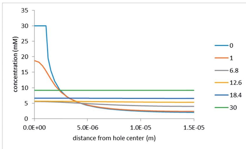
Fig. 6 Salt-concentration profiles in the horizontal direction at various distances (in  $\mu\text{m}$ ) from the mask/porous-medium interface as indicated in the legend: hole radius  $1 \mu\text{m}$ , inter-hole spacing  $30 \mu\text{m}$ , voltage drop  $200$  mV.
