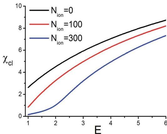
Fig. 5 The dependencies of the clenching coefficient for the athermal CS model of solid friction, eqn (35), on the applied electric field,  $\vec{E} = eEb/k_B T$ , for different concentrations of salt. The model parameters are  $\mu = 0.2$  and  $d = b$ , while the other parameters are the same as in Fig. 3. The magnitude of the normal force  $F_N$  is taken from the MD simulations.
