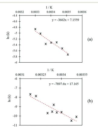
Fig. 8 Arrhenius plots corresponding to (a) the Cannizzaro reaction and (b) the catalytic oxidation of FF.
