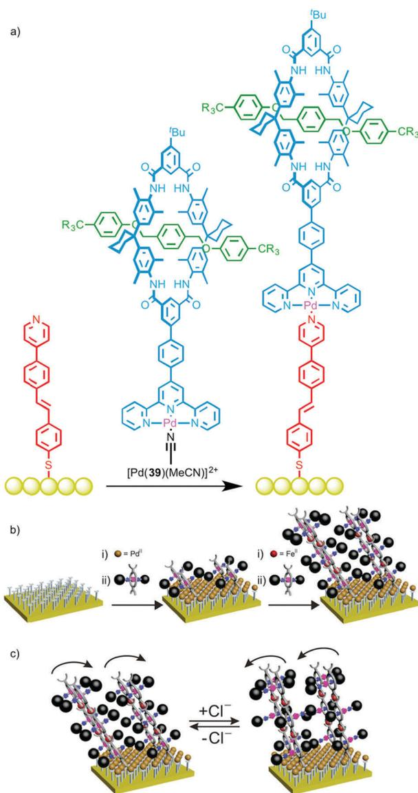
Fig. 21 (a) Schalley's rotaxane monolayer assembled using metallosupramolecular chemistry,<sup>57</sup> (b) a cartoon representation of the layer-by-layer deposition of Cl-responsive rotaxanes and (c) their proposed switching in the presence of Cl anions.<sup>58</sup> Adapted with permission from ref. 58. Copyright 2015 American Chemical Society.
