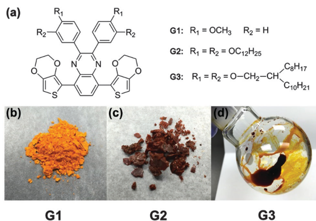
Fig. 1 (a) The molecular structure of G1, G2 and G3, (b), (c) and (d) the appearance of G1, G2 and G3 monomers, respectively.
