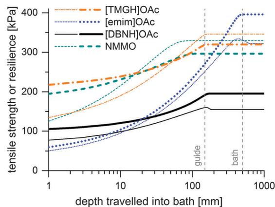
Fig. 4 Simulated minimum incipient filament strengths (thin lines) and resiliences (thick lines) at  $V_e = 0.05 \text{ ml min}^{-1}$  at  $D_R = 10$  in kPa as a function of distance travelled in a water bath.
