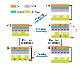
$\begin{tabular}{ll} Fig.~2 & Schematic illustration of the proposed working principle of the PPy NW-based TENG. \end{tabular}$
