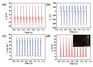
Fig. 3 (a) Short circuit current ( $l_{sc}$ ), (b) output voltage ( $V_o$ ), and (c) charge density ( $\sigma$ ) of the PPy NW-based TENG. (d)  $l_{sc}$  of the PPy NW-based TENG in one direction after rectification. The inset is the photograph of 372 commercial LEDs powered by the PPy NW-based TENG.
