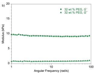
Fig. 7 Frequency-dependent dynamic shear measurements on (a) hPNB-PEO and (b) PCOD-PEO electrolytes. All membranes were plasticized with 32 wt% **PEG** 275 and had approximately 80 EO cross-linker units (88 for hPNB-PEO and 75 for PCOD-PEO), [1a]: [NB] or [1b]: [COD] ratios of 1:15, and [EO]: [Li] compositions of 20:15.
