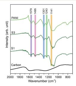
Fig. 2 Fourier transform infrared (FTIR) studies for the samples. FTIR spectra of carbon, PANI and carbon—PANI composites (samples S1 and S3).
