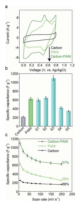
Fig. 4 Supercapacitor characterization. (a) Comparative CVs of carbon, PANI and carbon–PANI (composition S3) samples at a scan rate of 5 mV s<sup>-1</sup>. (b) Comparison of the specific capacitance performances of carbon, PANI and carbon–PANI nanocomposites (S1–S5) at various time intervals. (c) Variation of capacitance with scan rate for carbon, PANI and carbon–PANI nanocomposite (composition S3) samples.
