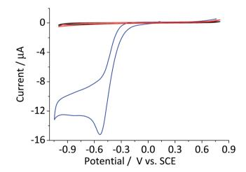
Fig. 3 Cyclic voltammetric curves of a bare glassy carbon electrode (red) and that modified with  $2.4 \times 10^{-5}$  g cm<sup>-2</sup> of hematite nanoparticles in N<sub>2</sub> saturated 20 mM KCl with 1.5 mM H<sub>2</sub>O<sub>2</sub> collected at the scan rate of 0.01 V s<sup>-1</sup>. Black line illustrates a cyclic voltammetric curve of bare glassy carbon in the same KCl solution without H<sub>2</sub>O<sub>2</sub>.
