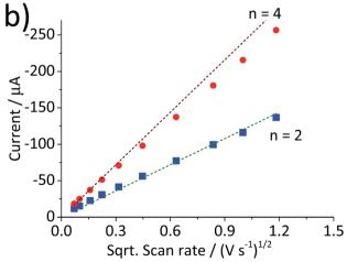
Fig. 2 (a) Cyclic voltammograms of a glassy carbon electrode modified with  $2.4 \times 10^{-5}$  g cm<sup>-2</sup> of hematite nanoparticles in O<sub>2</sub> saturated 20 mM KCl at the scan rate varied from 1.4 V  $s^{-1}$  to 0.005 V  $s^{-1}$ . (b) Plots of peak current as a function of the square root of the scan rate for the hematite modified electrode ( ) and for the bare electrode ( ). Dashed lines are calculated using eqn (5) for the 2-electron and the 4electron reactions.
