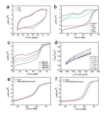
Fig. 5 (a) CV curves of the GMNCs in Ar-saturated and  $O_2$ -saturated 0.1 M KOH. (b) ORR polarization curves for the GMNCs, Pt/C, Mn<sub>3</sub>O<sub>4</sub>, MnO and GNCs at 1600 rpm. (c) ORR polarization curves of the GMNCs at different rotating speeds. (d) K–L plots of the GMNCs at different potentials. ORR polarization curves of the GMNCs (e) and Pt/C (f) before and after 10 000 potential cycles.
