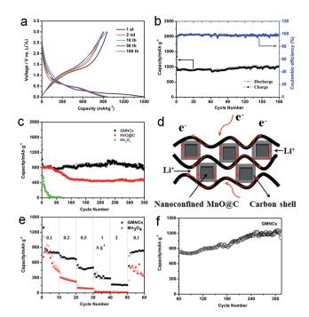
Fig. 4 (a) Discharge and charge profiles and (b) cycling performance of the GMNCs at 0.05 A  $\rm g^{-1}$ , (c) cycle performance of the GMNCs, MnO@C and Mn<sub>3</sub>O<sub>4</sub> at 0.1 A  $\rm g^{-1}$ , (d) schematic representation showing the paths for electrons and lithium-ions in the GMNCs. (e) Rate performance of the GMNCs and Mn<sub>3</sub>O<sub>4</sub> and (f) cycling performance of the GMNCs after 60 cycles rate measurement at 0.1 A  $\rm g^{-1}$ .
