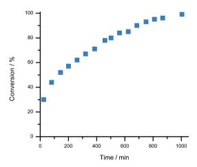
Fig. 3 Progress of  $H_2$  activation by 1[BArCl] in the presence of the mediator, BArF<sub>18</sub>.  $H_2$  (4 bar) was admitted to a sample of 1[BArCl] (0.028 mmol, 1.0 equivalents), BArF<sub>18</sub> (0.064 mmol, 2.3 equivalents), and 2,6-lutidine (0.048 mmol, 1.7 equivalents) in  $CD_2Cl_2$  and the formation of 1-H product was monitored using  $^1H$  NMR spectroscopy.
