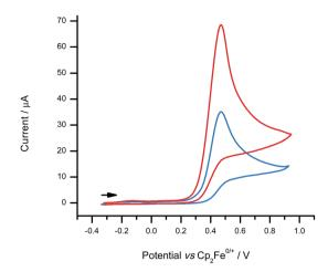
Fig. 4 CVs comparing the electrochemical behaviour of 1-H (1.8 mM) with (red line) and without (blue line) the addition of excess Brønsted base (2,6-lutidine; 6.7 mM) at a scan rate of 100 mV s<sup>-1</sup>.
