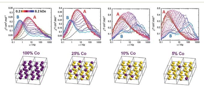
Fig. 23 Frequency dependent out-of-phase magnetic susceptibility ( $\chi''$ ) as a function of applied field (200–8200 Oe) at 2 K of [Co(DAPBH)(NO<sub>3</sub>)(H<sub>2</sub>O)] (67) magnetically diluted with [Zn(DAPBH)(NO<sub>3</sub>)(H<sub>2</sub>O)]. A and B represent two relaxation processes. Colour code: purple (Co) and yellow (Zn). Reprinted with permission from ref. 73. Copyright (2015) Royal Society of Chemistry.
