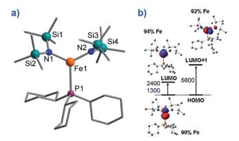
Fig. 10 (a) Molecular structure of [Fe(N(TMS)<sub>2</sub>)<sub>2</sub>(PCy<sub>3</sub>)], (TMS = SiMe<sub>3</sub>, Cy = cyclohexyl) (8). Colour code: orange (Fe), plum (P), teal (Si), blue (N), grey (C). Hydrogen atoms omitted for clarity. (b) TD-DFT calculated excited states and β-spin molecular orbitals (MOs). The energies of the excited states and the metal contribution to the MOs are also shown. Reprinted with permission from ref. 34. Copyright (2011) American Chemical Society.
