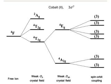
Fig. 7 Energy level diagram illustrating the effect of a weak octahedral crystal field and spin orbit coupling on the Co(II) ion as described in the text. Levels expanded for clarity. The multiplicity of states arising from spin—orbit coupling are given in brackets.
