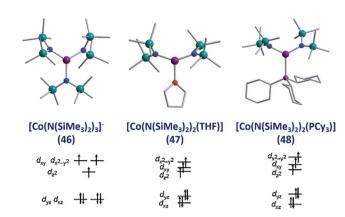
Fig. 19 Molecular structure and d-orbital splitting diagram for the three coordinate Co(II) complexes,  $[Li(15\text{-crown}-5)][Co\{N(SiMe_3)_2\}_3]$  (46),  $[Co\{N(SiMe_3)_2\}_2(THF)]$  (47) and  $[Co\{N-(SiMe_3)_2\}_2(PCy_3)]$  (48). Colour code: purple (Co), plum (P), teal (Si), blue (N), red (O), grey (C). Hydrogen atoms omitted for clarity. Adapted with permission from ref. 56. Copyright (2014) American Chemical Society.
