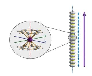
Fig. 5 A hypothesised chain-like arrangement of  $M(COT)_2$  monomers with uniaxial anisotropy, illustrating the concept of modular design of single-chain magnets. The axial anisotropy of each monomer is depicted as blue vectors and the vector addition of the monomeric axial anisotropies yields the net axial anisotropy (purple).
