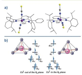
Fig. 16 (a) Molecular structures of [Co(LPh)(NCS)<sub>2</sub>] (25, left) and [Co(LMe)(NCS)<sub>2</sub>] (24, right). Colour code: purple (Co), blue (N), yellow (S), grey (C). (b) d-orbital splitting diagrams for 24 and 25, highlighting the effect of metal ion displacement from the basal plane. Reprinted with permission from ref. 47. Copyright (2011) American Chemical Society.
