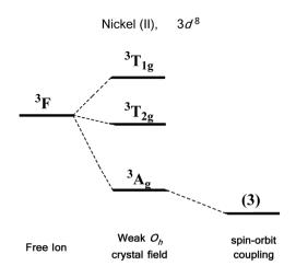
Fig. 6 Energy level diagram illustrating the effect of a weak octahedral crystal field and spin orbit coupling on the Ni(II) ion as described in the text. Levels expanded for clarity. The multiplicity of states arising from spin—orbit coupling are given in brackets.
