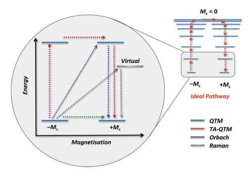
Fig. 2 Schematic representation of possible relaxation pathways in SMMs. Blue lines represent spin states. The grey line represents a virtual state by which Raman relaxation proceeds. Colour code: green = ground state QTM, red = thermally assisted QTM (TA-QTM), purple = Orbach relaxation, grey = Raman relaxation.
