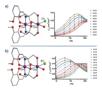
Fig. 15 Molecular structures of  $[Co^{II}Co^{II}(LH_2)_2(X)(H_2O)](H_2O)_4$  and the frequency dependence of the out-of-phase magnetic susceptibility collected in a 1000 Oe dc field. (a) X = Cl (21) and (b) X = Br (22). Colour code: purple (Co), bright green (Cl), light green (Br), blue (N), red (O), grey (C). Hydrogen atoms omitted for clarity. Reprinted with permission from ref. 44. Copyright (2014) American Chemical Society.
