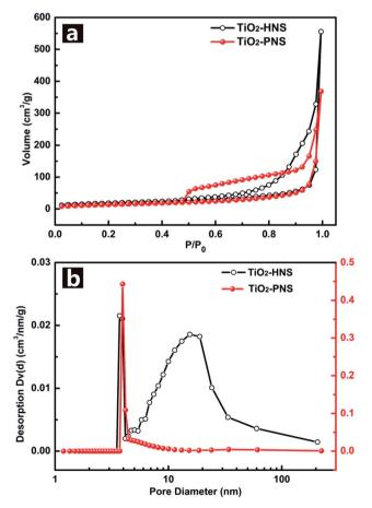
Fig. 3 (a) Nitrogen adsorption/desorption isotherms and (b) Barret–Joyner–Halenda (BJH) pore-size distribution curves of the  $TiO_2$ -HNSs and  $TiO_2$ -PNSs.
