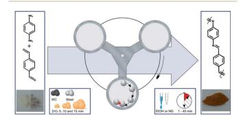
Fig. 1 The polycondensation reaction between p-benzoldicarbaldehyde and p-phenylenediamine conducted in a planetary ball mill can be controlled by milling material, ball size, milling time and addition of small amounts of solvent.
