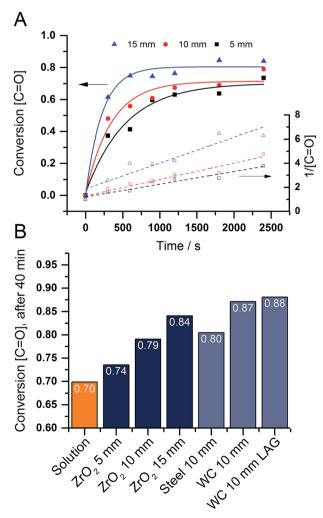
Fig. 3 (A) Conversion (full lines) and 2<sup>nd</sup> order rate law (dashed lines) in function of the zirconium oxide ball size. (B) Conversion after 40 minutes in function of different parameters. For detailed spectra see SFig. 10-15.†
