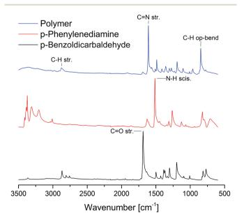
Fig. 2 IR spectra of the monomers and the polymer yielded by ball milling after 40 min with 10 mm ZrO<sub>2</sub> milling balls.
