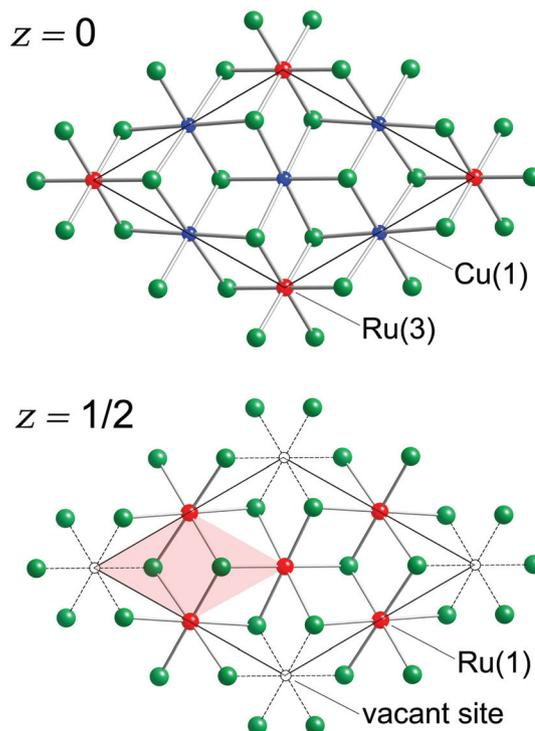
**Fig. 2** The *hcp* sub-lattice of Sb atoms in the  $\text{Cu}_3\text{Ru}_6\text{Sb}_8$  structure, shown as cut-outs at two different  $z$ -levels. Both projections are down the [001] direction. The Cu(1), Ru(1), and Ru(3) atoms forming slabs of fused octahedra are depicted. The vacant octahedral sites ( $1/8$  of all, shown as open circles) and the would-be NiAs sub-cell (shaded area) are also emphasized.
