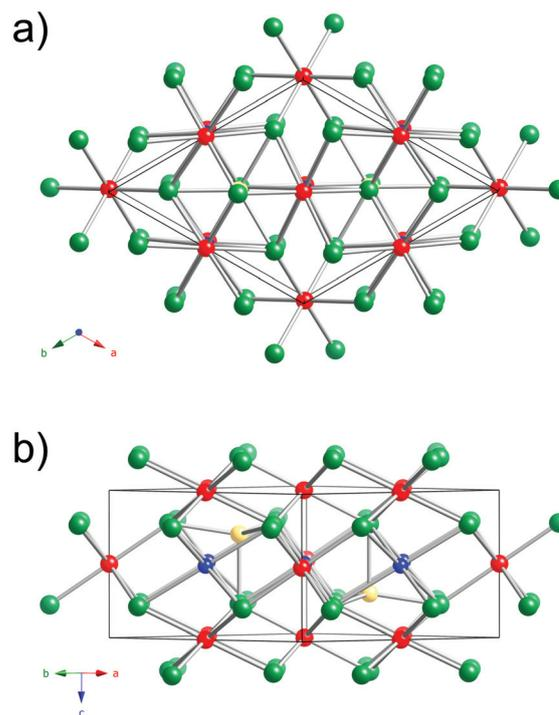
**Fig. 1** Two projections of the trigonal crystal structure of  $\text{Cu}_3\text{Ru}_6\text{Sb}_8$ , viewed down the [001] (a), and [110] (b) directions. The Sb atoms, arranged in a typical *hcp* fashion, are shown as green spheres. The Cu atoms and the Ru atoms filling octahedral holes are shown in blue and red, respectively. The Ru(2) atoms, which are (pseudo)tetrahedrally coordinated are drawn in yellow.
