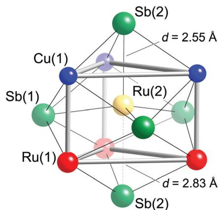
**Fig. 3** Schematic representation of the Ru(2) coordination. All atoms within 3  $\text{\AA}$  are drawn. The two Ru(2)–Sb(2) contacts that differentiate the structural description from tetrahedral to trigonal bipyramidal are emphasized.
