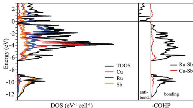
**Fig. 5** Left panel: Calculated total and partial density of states (DOS) curves for  $\text{Cu}_3\text{Ru}_6\text{Sb}_8$ . Right panel: Crystal Orbital Hamilton Population (COHP) curves for Ru–Sb and Cu–Sb interactions. Since the inverted COHP curves are shown, the positive and negative regions represent bonding and antibonding states, respectively. The Fermi level is the energy reference at 0 eV.
