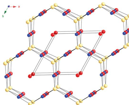
**Fig. 4** A schematic drawing of the metal-only substructure of  $\text{Cu}_3\text{Ru}_6\text{Sb}_8$ , viewed down the [001] direction. The Sb atoms are omitted. The Cu atoms are shown in blue, the Ru atoms filling octahedral holes (Ru(1) and Ru(3)) are drawn in red. The Ru(2) atoms are drawn in yellow.
