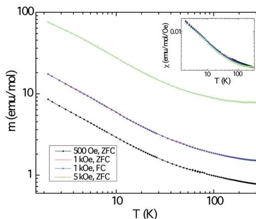
**Fig. 6** Temperature dependence of the magnetic moment  $m$  and the magnetic susceptibility ( $\chi = M/H$ , inset) of  $\text{Cu}_3\text{Ru}_6\text{Sb}_8$ , measured in zero field-cooled mode under applied fields of 500 Oe (black trace), 1000 Oe (red trace), and 5000 Oe (green trace). The blue trace represents the field-cooled data gathered under 1000 Oe.
