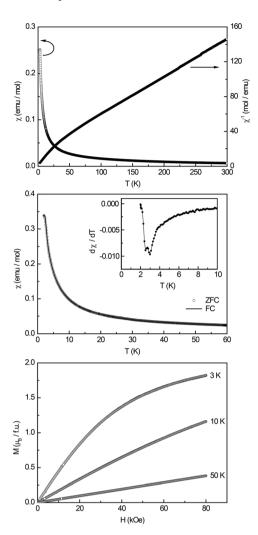
Fig. 6 Magnetic properties of Ce $_3$ Pt $_4$ Ge $_6$ : (top) Temperature dependence of the magnetic susceptibility  $\chi$  and its reciprocal  $\chi^{-1}$  measured with a magnetic field strength of 10 kOe; (middle) magnetic susceptibility in zero-field (ZFC) and field-cooled (FC) mode at 100 Oe; (bottom) magnetization isotherms at 3, 10, and 50 K.
