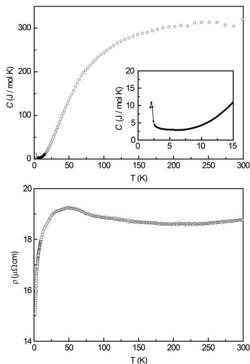
**Fig. 7** Physical properties of  $\text{Ce}_3\text{Pt}_4\text{Ge}_6$ : (top) Heat capacity measurement in the temperature range of 1.9–300 K, the inset shows the low temperature region between 1.9–15 K, indicating a  $\lambda$ -shaped anomaly; (bottom) temperature dependent electrical resistivity  $\rho$ .
