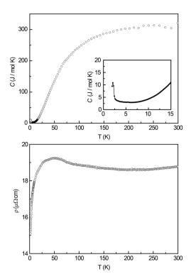
Fig. 7 Physical properties of  $Ce_3Pt_4Ge_6$ : (top) Heat capacity measurement in the temperature range of 1.9–300 K, the inset shows the low temperature region between 1.9–15 K, indicating a  $\lambda$ -shaped anomaly; (bottom) temperature dependent electrical resistivity  $\rho$ .
