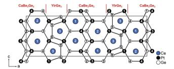
**Fig. 3** Extended unit cell of the commensurate supercell structure (Pnma, a=2618.26(14), b=441.33(2) and c=882.34(2) pm) of Ce<sub>3</sub>Pt<sub>4</sub>Ge<sub>6</sub>. The YIrGe<sub>2</sub> and CaBe<sub>2</sub>Ge<sub>2</sub> type parts are labelled. Ce atoms are depicted as blue, Pt atoms as black and Ge atoms as open white circles.
