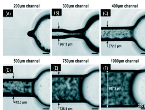
Fig. 11 (A–F) Micrographs of 500  $\mu\text{m}$  tall channels built in a range of widths. The actual width of each channels showed deviation of almost 30  $\mu\text{m}$  from design. The 300  $\mu\text{m}$  wide channel could only be partially cleared of resin, while the smaller channels did not clear at all and larger channels were fully cleared.<sup>60</sup> (Copyright 2015 RSC).
