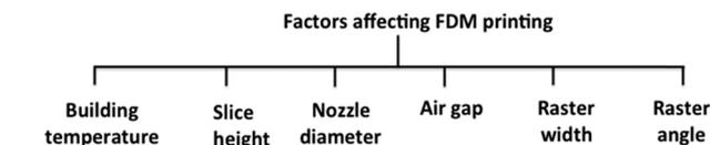
Fig. 18 Parameters affecting FDM process.
