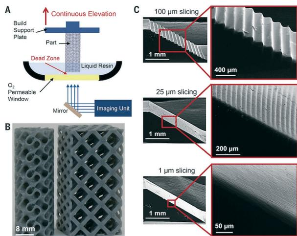
Fig. 13 (A) Schematic illustration of CLIP printer. (B–C) CLIP enables fast print speeds and layerless part construction.<sup>68</sup> (Copyright 2015 AAAS).
