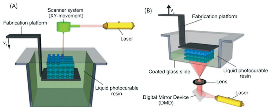
Fig. 7 Two SLA printing configurations. (A) Laser-scanning SL with the free surface/bath configuration. (B) DLP SLA with the constrained-surface/‘bat’ configuration.<sup>43</sup> (Copyright 2015 Elsevier).
