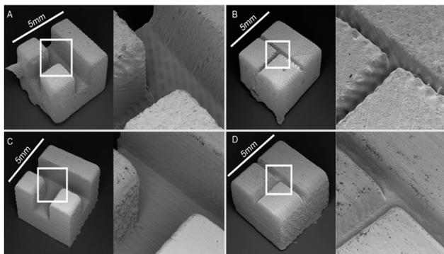
**Fig. 12** SEM images of open channels printed using the Form1+ (A and B) and Shapeways Frosted Ultra Detail (C and D). Each piece was designed to be 5 mm on a side. Channels were designed to be 1500 microns wide in A & C and 300 microns wide in B & D.<sup>61</sup> (Copyright 2015 Patrick *et al.*)
