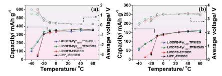
Fig. 6 Performance of Li/MCMB (a) and Li/LiFePO<sub>4</sub> cells (b) containing LiODFB-Pyr<sub>1,201</sub>TFSI/ES, LiODFB-Pyr<sub>1,201</sub>TFSI/DMS, LiODFB-EC/DEC or LiPF<sub>6</sub>-EC/DEC electrolytes at various temperatures with a current density of 0.1C
