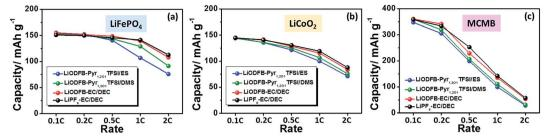
Fig. 7 Rate capability of the Li/LiFePO<sub>4</sub> (a), Li/LiCoO<sub>2</sub> (b) and Li/MCMB (c) cells with LiODFB-Pyr<sub>1,2O1</sub>TFSI/ES, LiODFB-Pyr<sub>1,2O1</sub>TFSI/DMS, LiODFB-EC/DEC or LiPF<sub>6</sub>-EC/DEC electrolytes.
