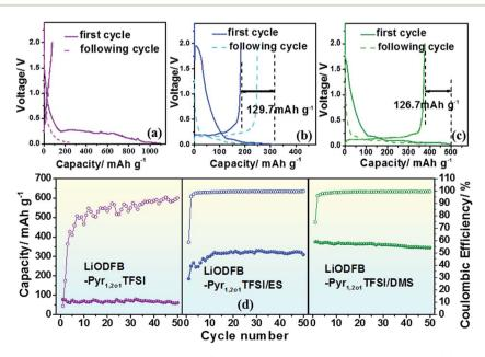
Fig. 3 First and subsequent charge and discharge curves of Li/MCMB cells with (a) LiODFB-Pyr<sub>1,201</sub>TFSI, (b) LiODFB-Pyr<sub>1,201</sub>TFSI/ES or (c) LiODFB-Pyr<sub>1,201</sub>TFSI/DMS electrolytes. (d) Cycling performance and coulombic efficiency of the cells with the three electrolyte samples.
