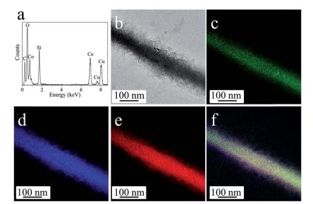
Fig. 2 (a) EDX spectrum taken from a single nanobelt, in which the C and Cu signals originate from the TEM grid. (b-f) EFTEM images: (b) zero-loss image, (c) Co L-edge, (d) Si L-edge, (e) O K-edge, (f) overlapping of Co, Si and O maps.
