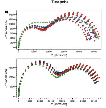
Fig. 7 (a) Current response from 300 mV applied potential to 14 (red) and 19 (blue) in a symmetric lithium metal cell. (b) AC impedance spectra collected during 24 hour operation of Li(s)|electrolyte|Li(s) symmetric cells. Top: Polymer 14. Bottom: Polymer 19. Red data represents impedance spectra taken without constant applied voltage. Blue data represents spectra taken with 300 mV applied voltage. Green data represents the final spectrum taken after the experiment.
