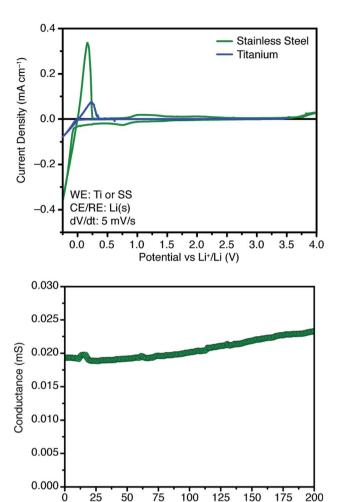
Fig. 5 Cyclic voltammograms of electrolyte 14 using titanium and stainless steel working electrodes at 90 °C (top), and time dependence of total conductance measured at room temperature in a symmetric Li(s)|electrolyte|Li(s) cell (bottom).
