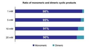
Fig. 2 Influence of substrate concentration on the formation of cyclodimers during the cyclization of 3 in 2:1 CH $_3$ CN/H $_2$ O (0.1 M oxalic acid) at 60 °C. The ratio was determined by HPLC at 220 nm as relative area% of depsi and amide products.
