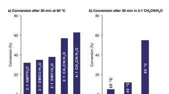
Fig. 1 Cyclization of 3: conversion determined by HPLC at 220 nm as relative area% of starting material 3 and products depsi-4 and amide-4 dependent on (a) solvents after 30 min at 60 °C in the presence of 0.1 M oxalic acid and (b) temperature in 2:1 CH<sub>3</sub>CN/H<sub>2</sub>O (0.1 M oxalic acid)
