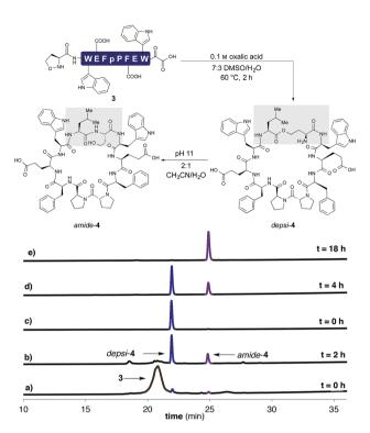
Scheme 2 Cyclization of 3 in 7 : 3 DMSO/H $_2$ O with 0.1 M oxalic acid at 60 °C after (a) 0 h (b) 2 h. (c) Purified depsi-4. (d) O,N-Acyl shift of depsi-4 at pH 11 in 2 : 1 CH $_3$ CN/H $_2$ O (200 mM phosphate buffer) after 4 h and (e) after 18 h.
