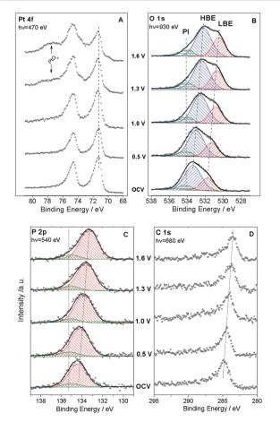
Fig. 2 Pt 4f (A), O 1s (B), P 2p (C), and C 1s (D) spectra acquired *in situ* under 0.3 mbar  $\rm H_2O$  and 180 °C at various cell voltages. Panels B and C also show the results of the O 1s and P 2p spectra deconvolution. See text for details.
