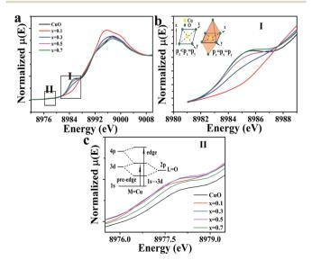
Fig. 3 (a) Normalized Cu–K edge XANES spectra for  $\operatorname{Cu_x Ir_{1-x}} O_\delta$  compositions. (b) Shows the shakedown transition and the inset is a diagram of the Cu-4p orbital energy in two different symmetries. (c) Shows the amplified pre-edge region and the inset diagram shows the energy level of possible transitions. (b) and (c) correspond to the selected areas. I and II. in (a).
