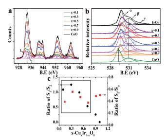
Fig. 4 (a) XPS spectra of Cu-2p in the Cu<sub>x</sub>lr<sub>1-x</sub>O<sub> $\delta$ </sub> compositions with x=0.1 de-convoluted; other compositions' de-convoluted spectra are shown in the ESI. (b) XPS spectra of O-1s in the Cu<sub>x</sub>lr<sub>1-x</sub>O<sub> $\delta$ </sub> compositions. (c) Pattern of the ratio of S<sub>1</sub>/S<sub>2</sub> and S<sub> $\beta$ </sub>/S<sub> $\alpha$ </sub> versus the doped amount x.
