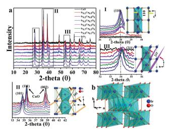
Fig. 2 (a) XRD patterns of the  $Cu_x Ir_{1-x}O_{\delta}$  compositions with different amounts of Cu doping. (I)–(III) correspond to the (a) selected areas. (b) Polyhedron picture of one  $IrO_2$  cell.
