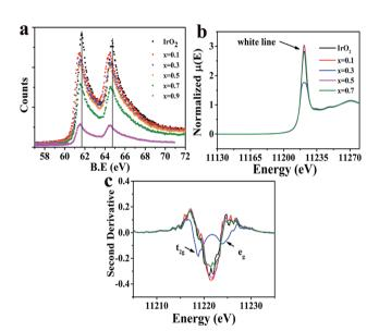
Fig. 5 (a) XPS spectra of Ir-4f in  $Cu_x Ir_{1-x}O_{\delta}$  compositions. The solid vertical lines correspond to the Ir-4f<sub>7/2</sub> and 4f<sub>5/2</sub> peak positions of IrO<sub>2</sub>. (b) Normalized Ir-L<sub>III</sub> edge XANES spectra for  $Cu_x Ir_{1-x}O_{\delta}$  compositions. (c) Second derivatives of Ir-L<sub>III</sub> edge XANES spectra for  $Cu_x Ir_{1-x}O_{\delta}$  compositions.
