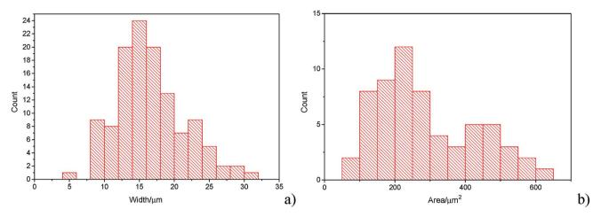
Fig. 3 (a) Histogram of widths of graphene nanoplatelets (b) histogram of area (assuming nanoparticles as rectangular platelets).
