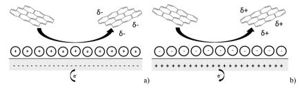
Fig. 1 Schematic diagram of the process postulated to occur during GNP impact where (a) the electrode is negative with respect to the PZC and (b) the electrode is positive with respect to the PZC.
