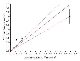
Fig. 7 Plot showing the average impact frequency–concentration relationship. The red line plotted indicates a diffusion coefficient of  $D_0 = 2 \pm 0.8 \times 10^{-13} \, \mathrm{m^2 \, s^{-1}}$  (error lines dashed). A linear relationship with respect to concentration is predicted by the integrated Szabo equation. All experiments are performed at +1.20 V in order to ensure a large capacitative signal for facile counting.
