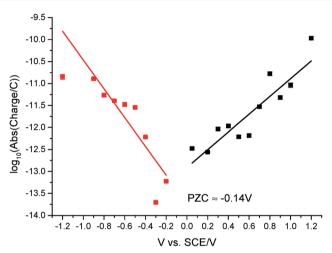
Fig. 6  $5.9 \times 10^{-13}$  mol dm<sup>-3</sup> suspension impacts with absolute charge of nanoparticle impacts in logarithmic (log<sub>10</sub>) scale plotted against applied potential (vs. SCE). Red squares: values with applied potential < 0 V; black squares: values with applied potential > 0 V (vs. SCE). The intersection potential of the two lines is used to estimate the PZC value of GNPs, where PZC is determined to be -0.14 V (vs. SCE).
