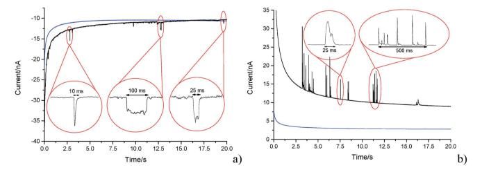
Fig. 4 Representative chronoamperometric scans in a  $5.9 \times 10^{-13}$  mol dm<sup>-3</sup> suspension using a cylindrical carbon fibre wire electrode at a potential of (a) -1.20 V (vs. SCE); (b) +1.20 V (vs. SCE). Blue line: blank scan in 0.1 M KCl with 50 mM KH $_2$ PO $_4$ , 50 mM K $_2$ HPO $_4$  (PBS) buffer solution mentioned in the Experimental section. Black line:  $5.9 \times 10^{-13}$  mol dm $^{-3}$  graphene nanoplatelet (GNP) suspension scan showing capacitative impacts
