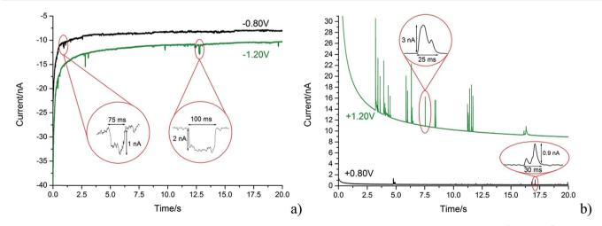
Fig. 5 Comparison of spike sizes at different potentials from representative chronoamperometric scans in a  $5.9 \times 10^{-13}$  mol dm<sup>-3</sup> suspension using a cylindrical carbon fibre wire electrode. Smaller features at lower applied potential (vs. SCE) magnitude can be seen. (a) Black line: -0.80 V (vs. SCE). Green line: -1.20 V (vs. SCE). (b) Black line: +0.80 V (vs. SCE). Green line: +1.20 V (vs. SCE).
