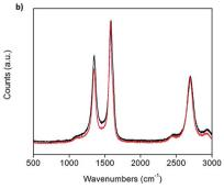
Fig. 1 (a) X-ray powder diffraction of 46 wt% Pt-CNTs (red) along with a reference trace<sup>25</sup> (black), and (b) Raman spectra of as-received (red) and 46 wt% Pt-decorated (black) commercial CNTs showing that the carbon nanotube structure is largely unchanged after decoration.
