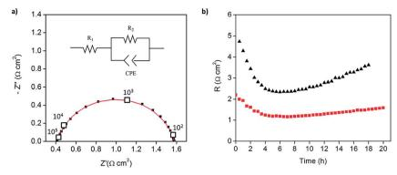
Fig. 7 Symmetric cell impedance measurements Pt-CNT based electrodes prepared by strategy 2: (a) Nyquist plot for 46 wt% Pt-CNT-CsH<sub>2</sub>PO<sub>4</sub> composite after 4 hours (inset: equivalent circuit used for fitting) and (b) temporal evolution of the electrode resistance values of 30 wt% (black) and 46 wt% (red) Pt-CNT-CsH<sub>2</sub>PO<sub>4</sub> composites, showing higher stability in the electrolyte with higher Pt loading.
