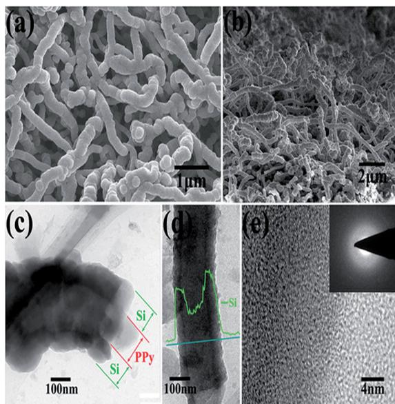
Fig. 8 (a) and (b) top and cross-sectional SEM images of PPy–Si core–shell nanofiber network after Si deposition. (c) and (d) TEM images of the core–shell structure of Si@PPy nanocables. (e) High-resolution TEM image of Si coatings. Inset of (e) SAED image of Si coatings (reprinted with permission from ref. 186, copyright 2012, Royal Society and Chemical Journal).
