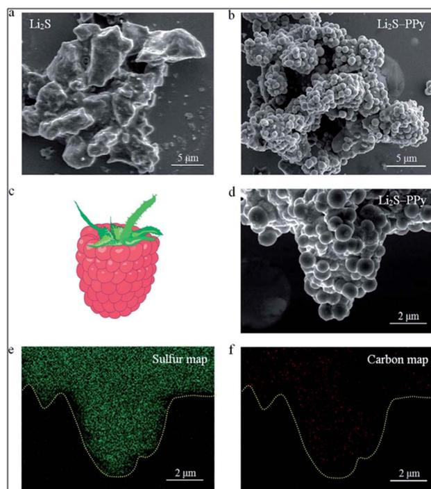
Fig. 11 SEM images of (a) pristine  $\text{Li}_2\text{S}$  particles and (b) as-synthesized  $\text{Li}_2\text{S}$ -PPy composite structures. (c) Schematic of a raspberry and (d) SEM image of a representative  $\text{Li}_2\text{S}$ -PPy raspberry-like composite together with the corresponding elemental maps for (e) sulfur and (f) carbon (reprinted with permission from ref. 246, copyright 2014, Royal Society and Chemical Journal).
