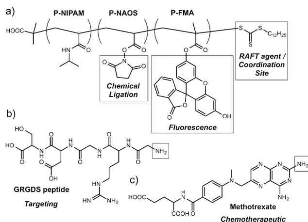
**Fig. 9** (a) Chemical structure of the RAFT random co-polymer, comprised of *N*-isopropylacrylamide (NIPAM), *N*-acryloxysuccinimide (NAOS), and fluorescein-*O*-methacrylate (FMA) monomers, used to coat  $[\text{Gd}(1,4\text{-bdc})_{1.5}(\text{H}_2\text{O})_2]_n$  nanoparticles. The activated NHS ester allows post-synthetic conjugation of (b) targeting GRGDS peptides and (c) methotrexate chemotherapeutic units through reaction with free amino groups.
