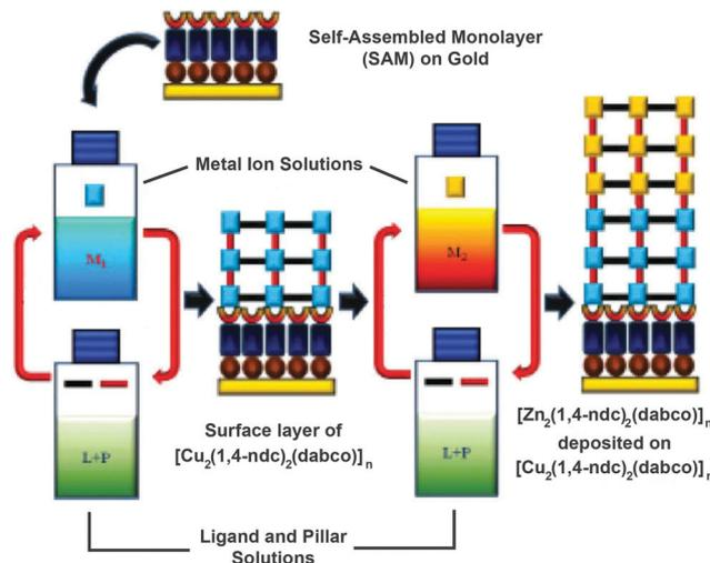
Fig. 21 Mechanism for the preparation of an epitaxial MOF thin film of [Zn<sub>2</sub>(1,4-ndc)<sub>2</sub>(dabco)]<sub>n</sub> deposited on [Cu<sub>2</sub>(1,4-ndc)<sub>2</sub>(dabco)]<sub>n</sub> in a layer-by-layer deposition approach on a self-assembled monolayer. Adapted from ref. 74 with permission from The Royal Society of Chemistry.
