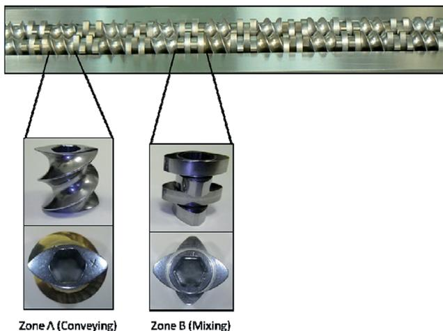
Fig. 4 Typical twin extrusion configuration used for the formation of cocrystals. The conveying and mixing zones are shown. Typical output rate is approximately  $0.5 \text{ g min}^{-1}$ . PXRD suggests comparable properties for the product to that obtained by conventional solution growth. The possibility of simultaneously blending the cocrystal product within a polymer matrix is an important additional advantage of the method. Reproduced from ref. 58.
