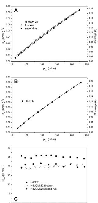
Fig. 7 (A) Adsorption isotherm of CO on H-MCM-22 (Si: Al = 24.5:1) at 303 K; (B) adsorption isotherm of CO on H-FER zeolite (Si: Al = 27.5:1) at 303 K; (C) adsorption heat of CO on H-FER (squares) and H-MCM-22 (circles) measured by calorimetry at 303 K, as a function of coverage.
