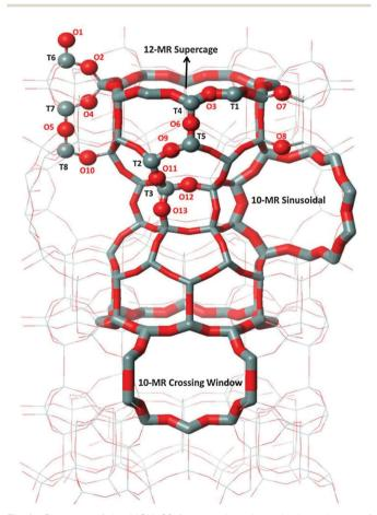
Fig. 1 Structure of the MCM-22 framework and numbering scheme of the eight non-equivalent T sites and thirteen non-equivalent framework oxygen atoms. Framework T sites and framework oxygen atoms are depicted in grey and red, respectively.
