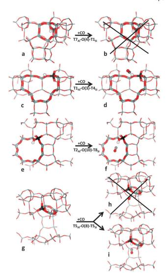
Fig. 3 Brønsted-acid sites without and with an adsorbed CO (left and right parts, respectively) shown for Al in T7 (a, b), T1 (c, d), T2 (e, f), and T5 (g–i). Framework Si, Al, and O atoms are depicted in grey, black, and red colour, respectively, while the H atom of the Brønsted-acid OH group, and C and O atoms of CO are depicted as white, grey, and red balls, respectively.
