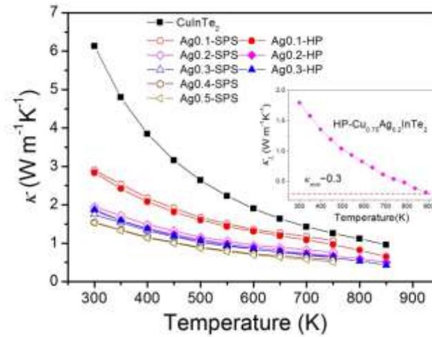
Fig. 10. Temperature dependence of thermal conductivity for  $\text{Cu}_{1-x-\delta}\text{Ag}_x\text{InTe}_2$  ( $x = 0 - 0.5$ ). The inset picture displays lattice thermal conductivity  $\kappa_L$  of  $\text{HP-Cu}_{0.75}\text{Ag}_{0.2}\text{InTe}_2$ . At 886 K, the value of  $\kappa_L$  hits the  $\kappa_{min}$ .
