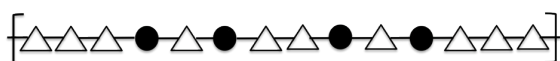
Figure 7. Hypothesized monomer distribution scheme in the copolymer for P(DAA- co -AEMA). Solid circle, DAA- p ; empty triangle, AEMA.
