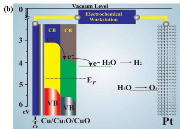
Fig. 5 (a) Photoelectrochemical response of the \text{Cu}/\text{Cu}_2\text{O}/\text{CuO} photoelectrode under illumination of chopped AM 1.5G. The inset shows the photocurrent density decay for the electrode held at 0V vs RHE under chopped light illumination. (b) Proposed energy band diagram of the \text{Cu}/\text{Cu}_2\text{O}/\text{CuO} composite electrode. 45 Copyright 2012 The Royal Society of Chemistry.
