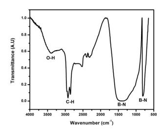
Figure 7. FTIR spectrum of h-BN foam after the burning of absorbed oil.
