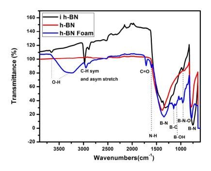
Figure 3. FTIR spectra of h-BN, i-hBN and h-BN foam, comparing the functionalities of h-BN foam with pure h-BN powder and functionalised h-BN.
