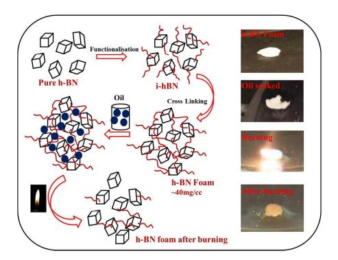
Figure 6. Schematic of the h-BN foam development and its oil adsorption and burning. Real time images of the oil (used engine oil) soaking and later burning of the foam are shown on the right.
