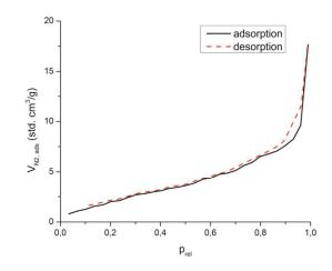
Figure 5. The adsorption-desorption isotherm pairs of h-BN foam.
