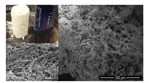
Figure 1. (A) Photograph of h-BN foam. The size of the foam is shown *via* the adjacent scale. (B) and (C) are the FESEM images of the same foam showing the microscopic structure of the h-
