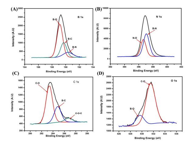
Figure 4. Deconvoluted XPS Spectra: (A) B 1s (B) N 1s (C) C 1s and (D) O 1s of 3D h-BN foam.
