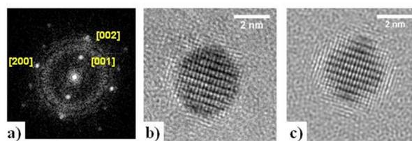
**Fig. 1.2:** a) Fourier transform of the experimental HRTEM image of a CoPt cluster where the chemical L1<sub>0</sub> order is visible. (b). The [001] peak is the signature of the chemical order in the nanoparticle. c) Simulated HRTEM image of a perfectly ordered cluster.
