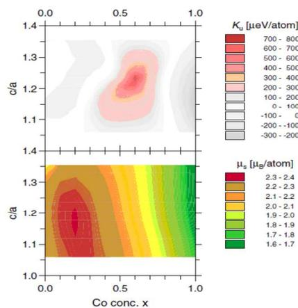
**Fig. 2.5:** (color). Calculated effective anisotropy  $K_u$  (upper panel) and saturation magnetic moment  $\mu_s$  (lower panel) of tetragonal  $\text{Fe}_{1-x}\text{Co}_x$  as a function of the  $c/a$  ratio and the Co concentration  $x$ , from ref<sup>62</sup>.
