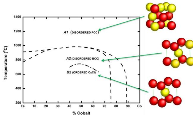
**Fig. 2.4:** Bulk FeCo Phase diagram adapted from ref<sup>61</sup>
