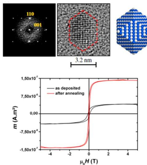
**Fig. 2.1:** Evidence of B2 phase from HRTEM observation obtained on annealed FeRh of 3 nm NPs (top). Hysteresis loops at 2 K obtained on 3 nm FeRh NPs showing the FM order and the global magnetization enhancement upon annealing (bottom)
