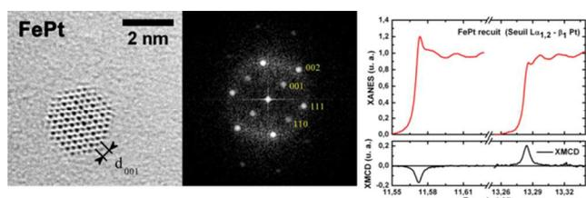
**Fig. 1.5:** Experimental HRTEM image and corresponding Fourier transform obtained on a FePt cluster where the chemical  $L1_0$  order is visible (left). Evidence of induced magnetic moment in Pt from XMCD measurement at  $L_{2,3}$  Pt edge (right).
