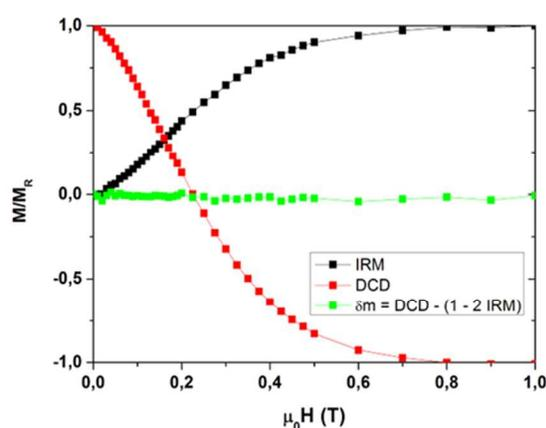
**Fig. 1.3:** IRM( $H$ ), DcD( $H$ ) and  $\delta m$  for annealed CoPt clusters embedded in an amorphous carbon matrix. The values presented here are divided by the remanent magnetization ( $M_R = \text{IRM}(\infty)$ ).
